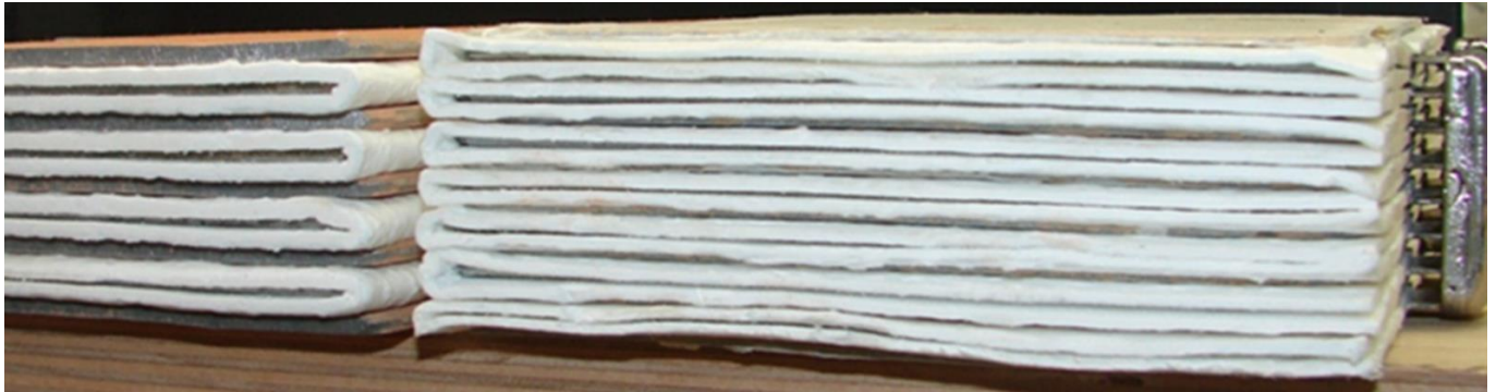
Figure 2: Comparison of plate stack AGM (classic) vs. pure lead design (grid | Xtreme VR) at same volume
