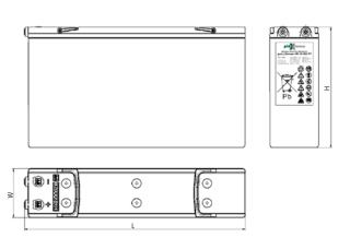
Tightening torque of terminal screw: 15 Nm - 133 lbf in
