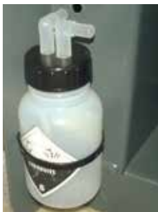
Figure 7: Condensate separator fixed to the carrier
