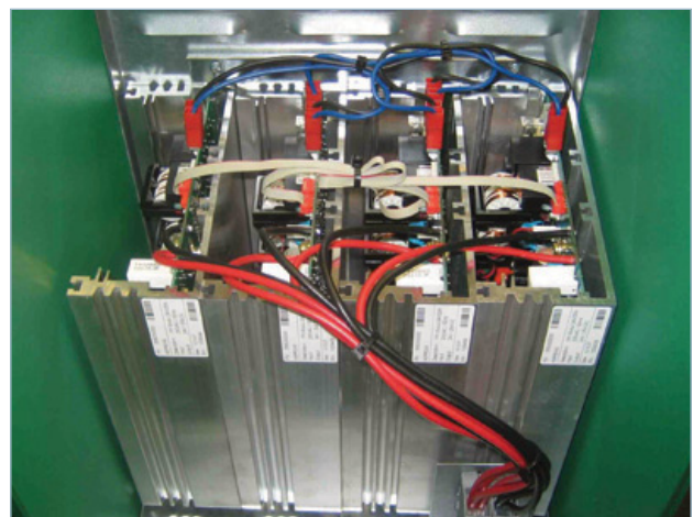
Parallel connected power modules, charger open
